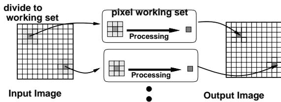
**Figure 1. The parallel image processing working set**
