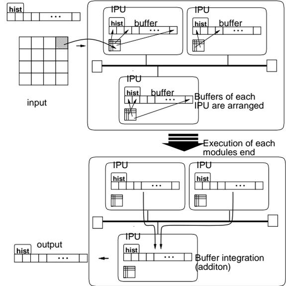
Figure 3. Histogram calculation using programmable global variable buffer
