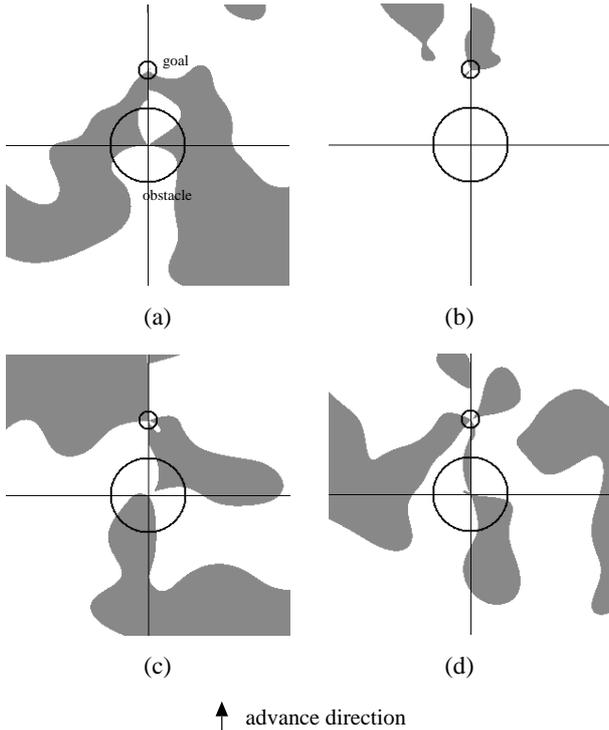
Figure 7: The example of construction of the state space in each action: (a)  $a_1$  (advance), (b)  $a_2$  (retreat), (c)  $a_3$  (left rotation), (d)  $a_4$  (right rotation)
