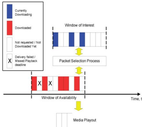
Figure 3 : Data buffer for PALMS-SP node
