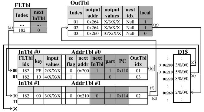
Fig. 8. Input matching flow on expanded MemoTbl.
