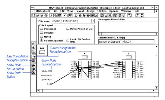
Fan-in and fan-out lines are updated automatically when you move an assignment. In addition, if you move a node to a new location, the assignment color changes if the **Show Moved Nodes in Gray** command (Options menu) is turned on.
