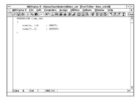
The ports enable and clk are inputs, and the ports time[7..0] are outputs, of time\_cnt.tdf.
