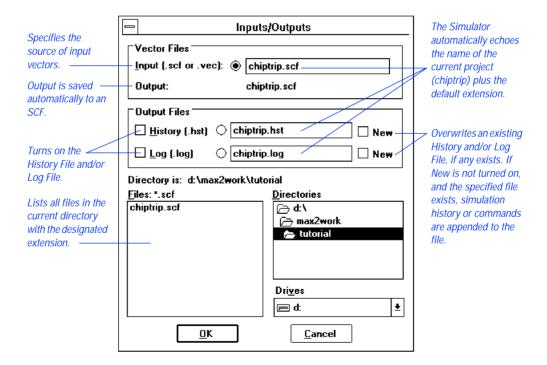
The simulation input file **chiptrip.scf** appears in the *Input* (*.scf or .vec*) box under *Vector Files*. If you want to use a Vector File or SCF with a name other than the project name, you must specify the filename in this box.
