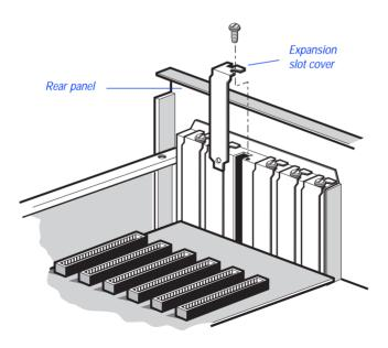
5. Insert the card into the expansion slot and fasten the retaining bracket with the screw from the slot cover. See Figure 1-6.
