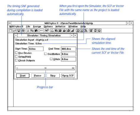
To simulate a project, you must first compile it and instruct the Compiler to generate a Simulator Netlist File (.snf) for functional, timing, or linked multi-project simulation. The functional, timing, or linked SNF for the current project is then loaded automatically when you open the Simulator.
