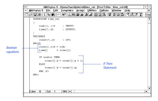
If the enable signal is high, the If Then Statement assigns the value count[].q + 1 to count[].d; if enable is low, count[].d remains unchanged.
