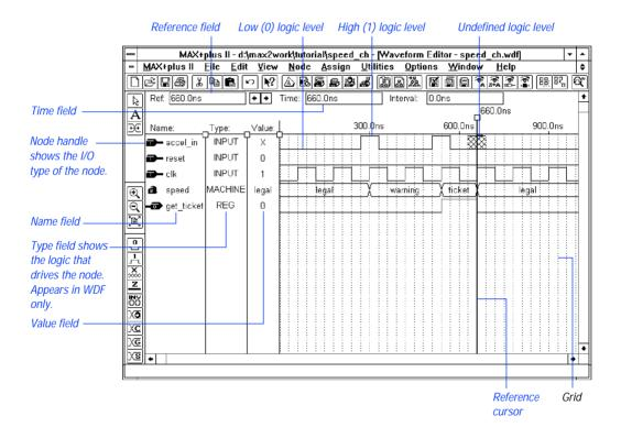
Waveform design entry offers an alternative to graphic and text design entry. You create a waveform design by specifying combinations of input logic levels and desired outputs as graphical waveforms. A WDF can contain both logical and state machine inputs, as well as combinatorial, registered, and state machine outputs. Buried nodes can also be used to help define desired outputs.
