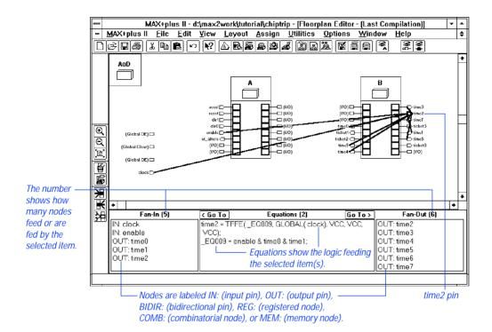
If the Show Node Fan-In and Show Node Fan-Out commands (Options menu) are turned on, the Floorplan Editor displays the fan-in and fan-out lines that correspond to the items listed in the Report File Equation Viewer window
