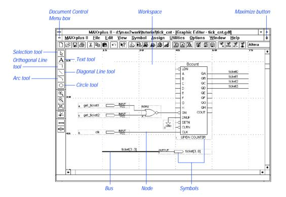
The Graphic Editor is a sophisticated schematic capture program that allows you to enter even complex designs quickly and easily. The extensive primitive, megafunction, and macrofunction libraries—including the Library of Parameterized Modules (LPM)—provide basic building blocks for constructing a design, while the symbol-generation capability lets you build your own libraries of custom functions.
