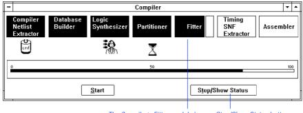
The Compiler's Fitter module is currently processing the project.
