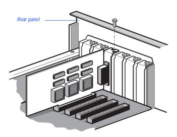
6. Tighten all the locking screws on all connectors.
