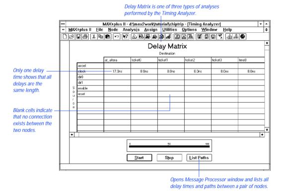
The Timing Analyzer uses the network and timing information from a timing Simulator Netlist File (.snf) generated by the Compiler. The Timing Analyzer can also use a linked SNF that links the timing SNFs of other projects.
