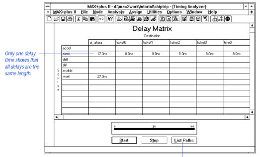
Opens Message Processor window and lists all delay times and paths between a pair of nodes.
