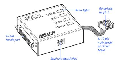
Figure 1-12. BitBlaster and 10-Pin Female Connector
