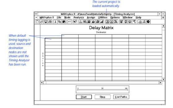
The Timing Analyzer automatically "tags" all input pins as timing sources and all output pins as timing destinations for Delay Matrix analysis. The names of nodes with this "default timing analysis tagging" are not visible until after the analysis is run. Each of the three analysis modes has its own display and appropriate default timing analysis tagging for nodes.
