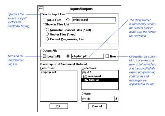
2. If necessary, turn on the *Log* (*.plf*) option under *Output File*. The filename chiptrip.plf appears automatically in the *Log* (*.plf*) box.
