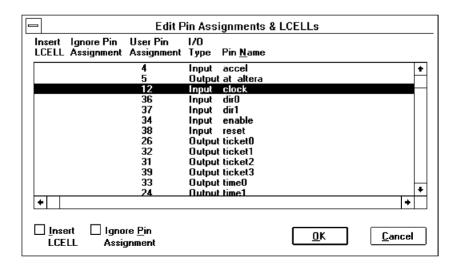
b. Turn on the *Ignore Pin Assignment* option at the bottom of the dialog box.
