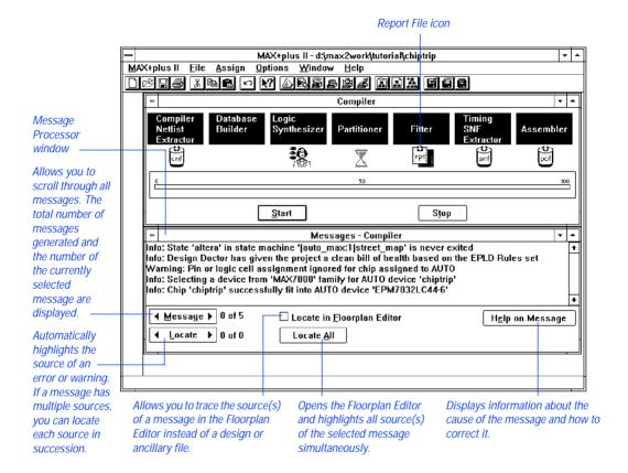
As shown in the illustration, the Design Doctor has given the **chiptrip** project a "clean bill of health," and the Compiler has selected the EPM7032LC44-6 device (an EPM7032-6 device in a 44-pin plastic J-lead chip carrier package) for the project.
