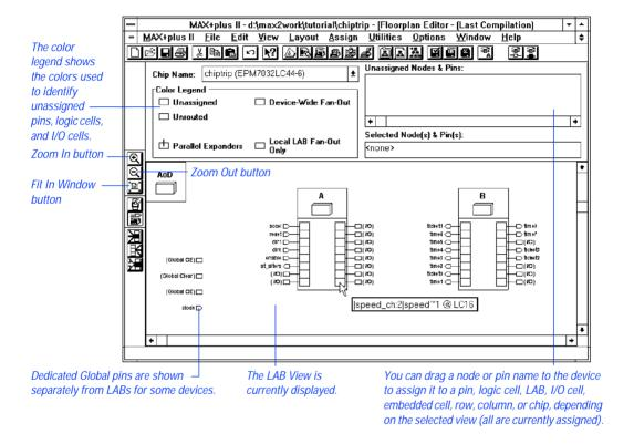
The Floorplan Editor provides a convenient method to enter and edit physical device resource assignments for your project. Two displays are available:
